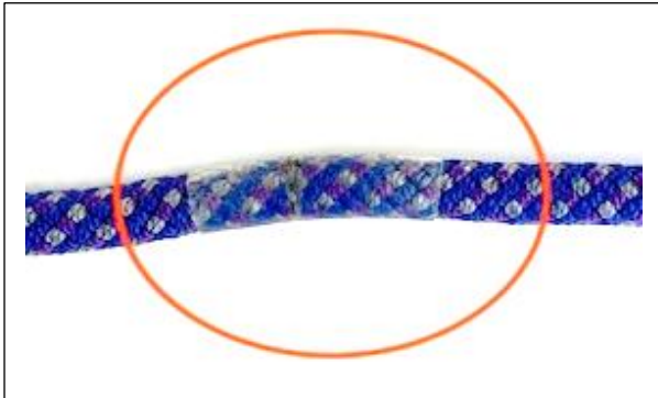
Splice with transparent heat shrink.
