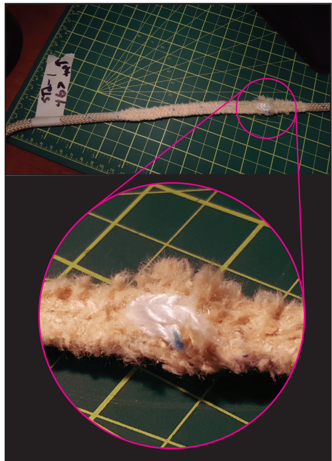
Core shot SafeTech sample after abrasion testing.
