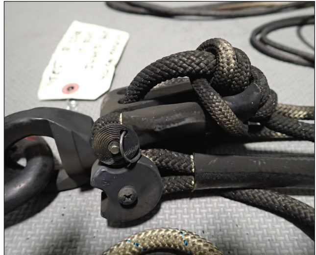
Damage to AZTEK Kit cause by exposure to arc flash testing.
